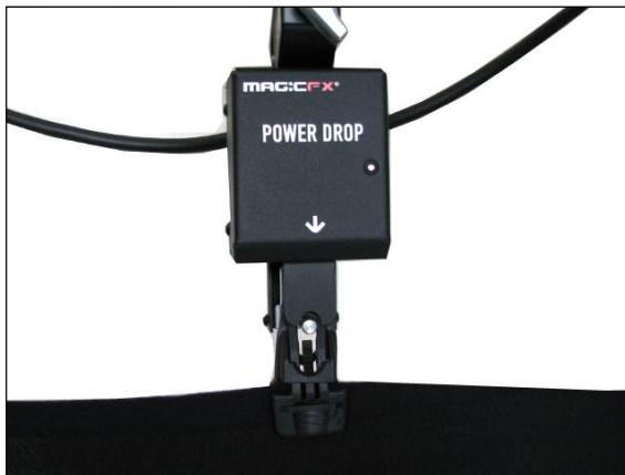
Then push the opening of the curtain clamp over the drop pin of the Power Drop and click this to a closed position as described in step 7.
